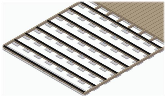
Joist tape used between decking and joists.
