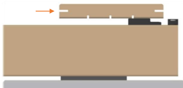
Figure 3: Fit the board on the substructure and press the lips into the holders.
