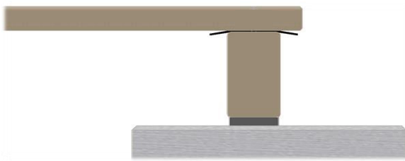
Example of use of a moisture barrier. Spacer block between concrete slab and joist. Suitable sill tape between joist and decking.
