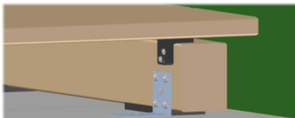
Figure 8: Screw the end clip to the substructure.
