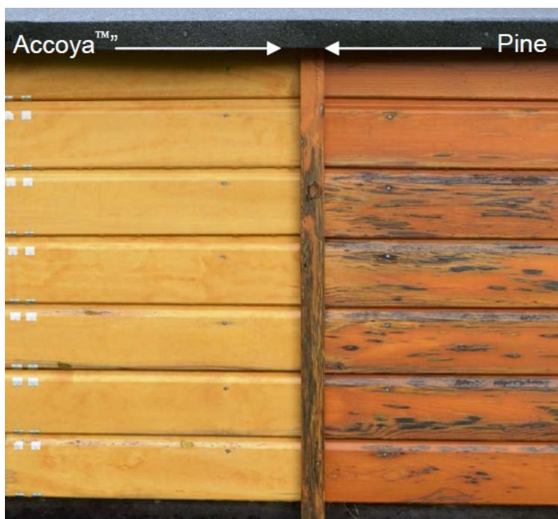
Test set-up after 7 years of exposure in January 2015
