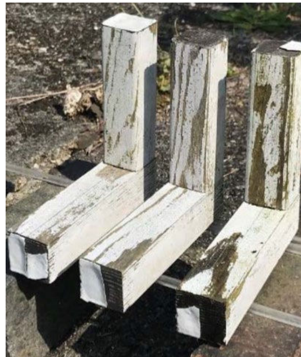
The acetylated L-joints after 20 years of exposure
