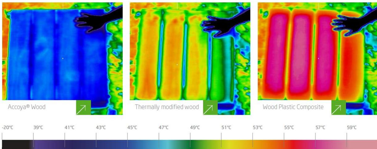
*Figure 10: Thermogram images of Accoya, thermally modified wood and WPC.*
